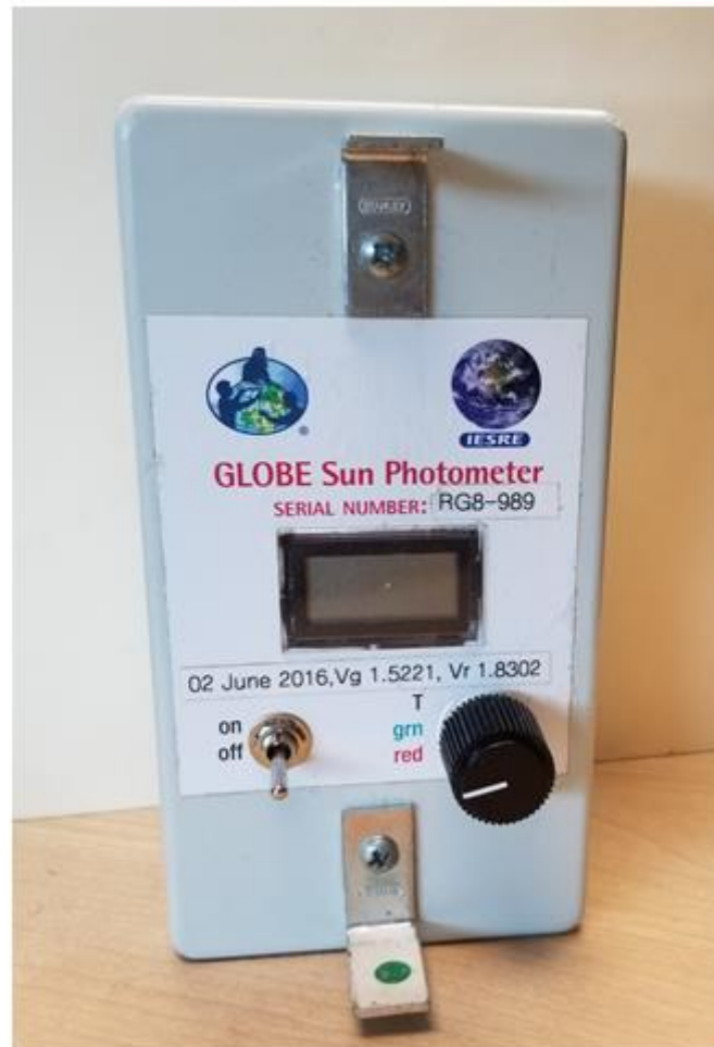
Figure 2. The GLOBE hand held sun photometer. The GLOBE sun photometer has two channels, green light at wavelength 505nm and red light at wavelength 625nm.
